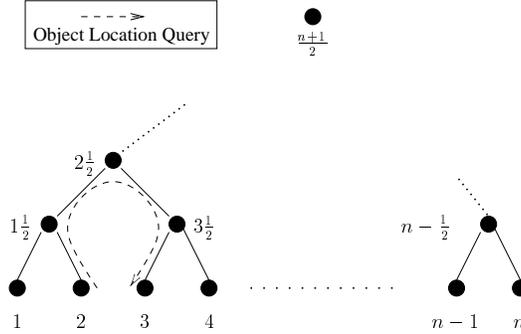
Figure 1: A *perfect base-2 Tapestry tree, with hypothetical average parents*.. A sample object location query with a stretch of three is shown.
